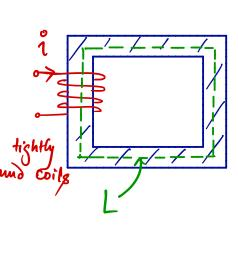
· Consider an iron piece with a cross piece with a cross sectional area A, and an average length around the loop being L as shown. as shown.
